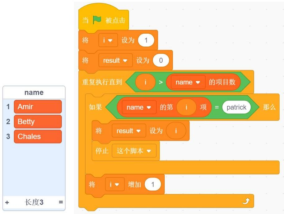
The image shows a Scratch script and a data table. The table has a header 'name' and three rows: 1 Amir, 2 Betty, 3 Chales. The script starts with 'When green flag is clicked', sets 'i' to 1 and 'result' to 0. It enters a 'Repeat until' loop with condition 'i > name's item count'. Inside, an 'if' block checks 'name's i-th item = patrick'. If true, it sets 'result' to 'i' and stops the script. If false, it increments 'i' by 1.
